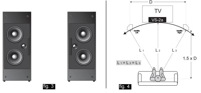
For digital 5.1-channel surround systems, we recommend that all five speakers be placed equidistant from the listening position. For Dolby Pro-Logic® systems, it is preferable to have a more diffuse, ambient sound radiating from behind the listening position. This is accomplished by placing the rear (surround) speakers so that they fire across the room at each other (not directly toward the seating position), and by placing them 3 to 4 feet above ear level.
